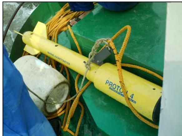
The Sensor of Proton-4 magnetometer
