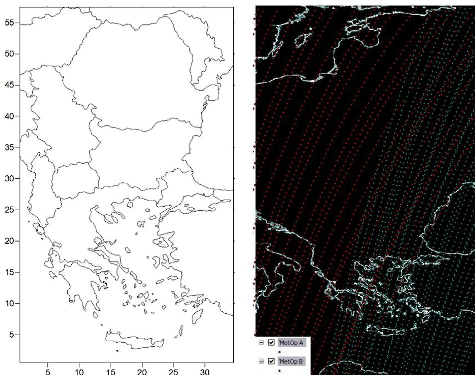
Fig. 5. The Balkan domain of BgCWFS (left) and the corresponding area covered by one track of *MetOp A* (blue dots) and one of *MetOp B* (red dots) satellites with pointed centres of their measurement cells (right)
