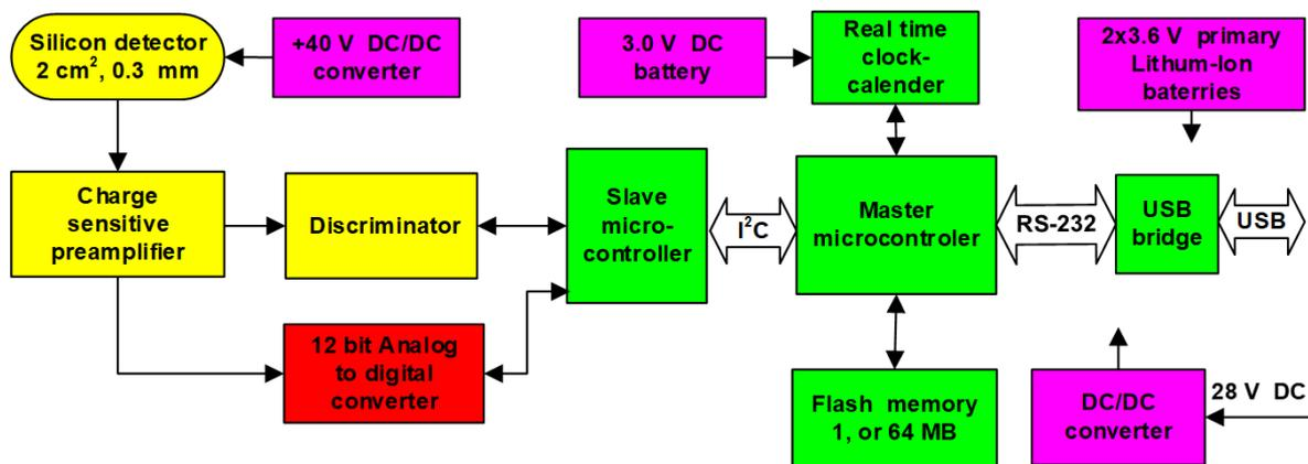
Fig. 1. Unified block-diagram of the three Liulin spectrometers
